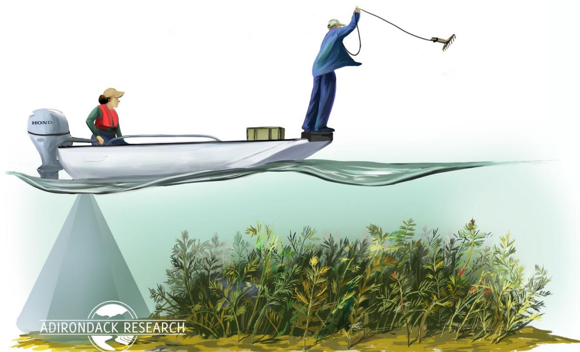
Figure 1: Illustration of the survey techniques utilizing a combination of sonar recording and manual rake toss.
